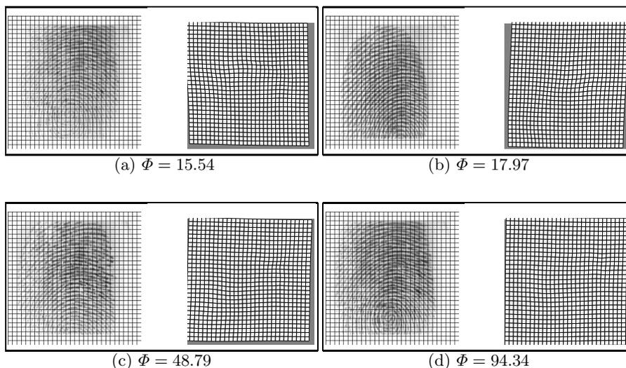
**Fig. 2.** The average deformation model (shown as deformations on a reference grid) corresponding to 4 templates of a finger sorted in increasing  $\Phi$ -values. (a) is chosen to be the optimal template since it has the least  $\Phi$ -value.
