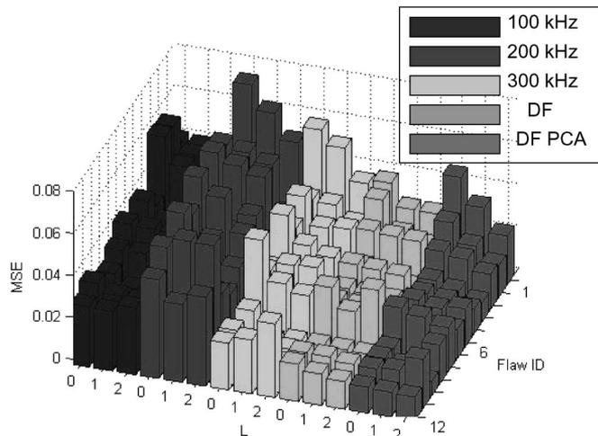
Fig. 6. MSE between the PME of the posterior pdf and the true profiles versus the state vector length parameter  $L$  at different measurement modes for experimental data.
