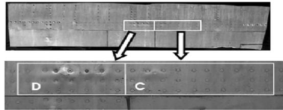
Fig. 8. Aircraft lap joint specimen.
