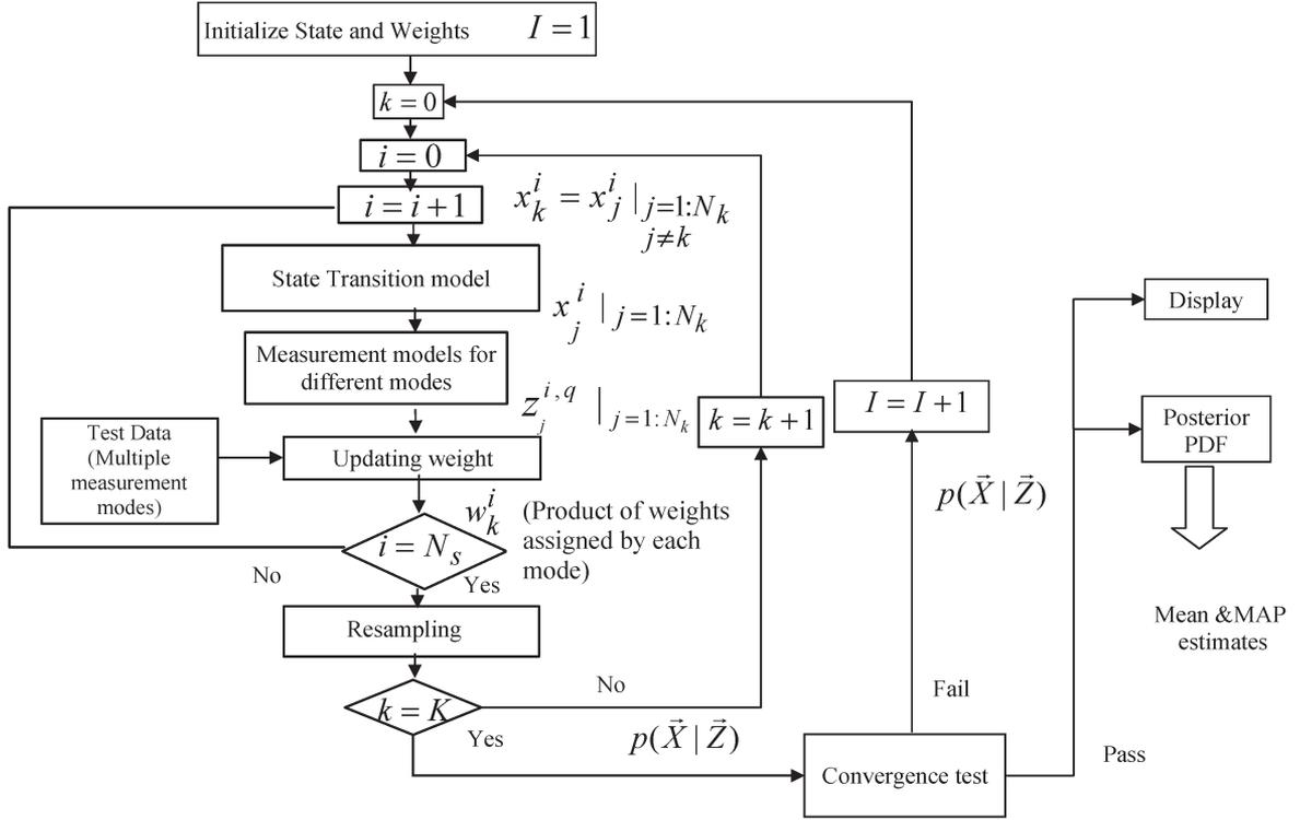
Fig. 3. Particle filter implementation for flaw profiling.
