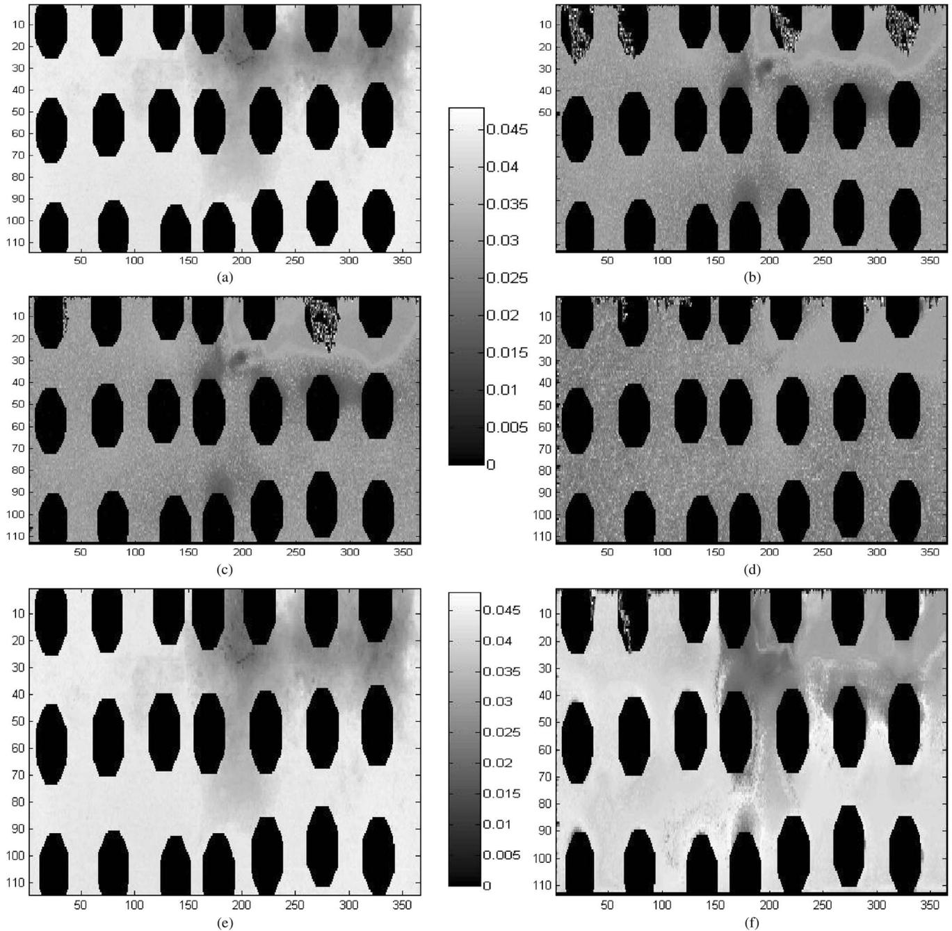
Fig. 9. Inversion results of specimen C (data fusion). (a) and (e) True profile. (b)–(d) and (f) Predicted profiles using ET data at 5.5, 17, 30 kHz and data fusion.
