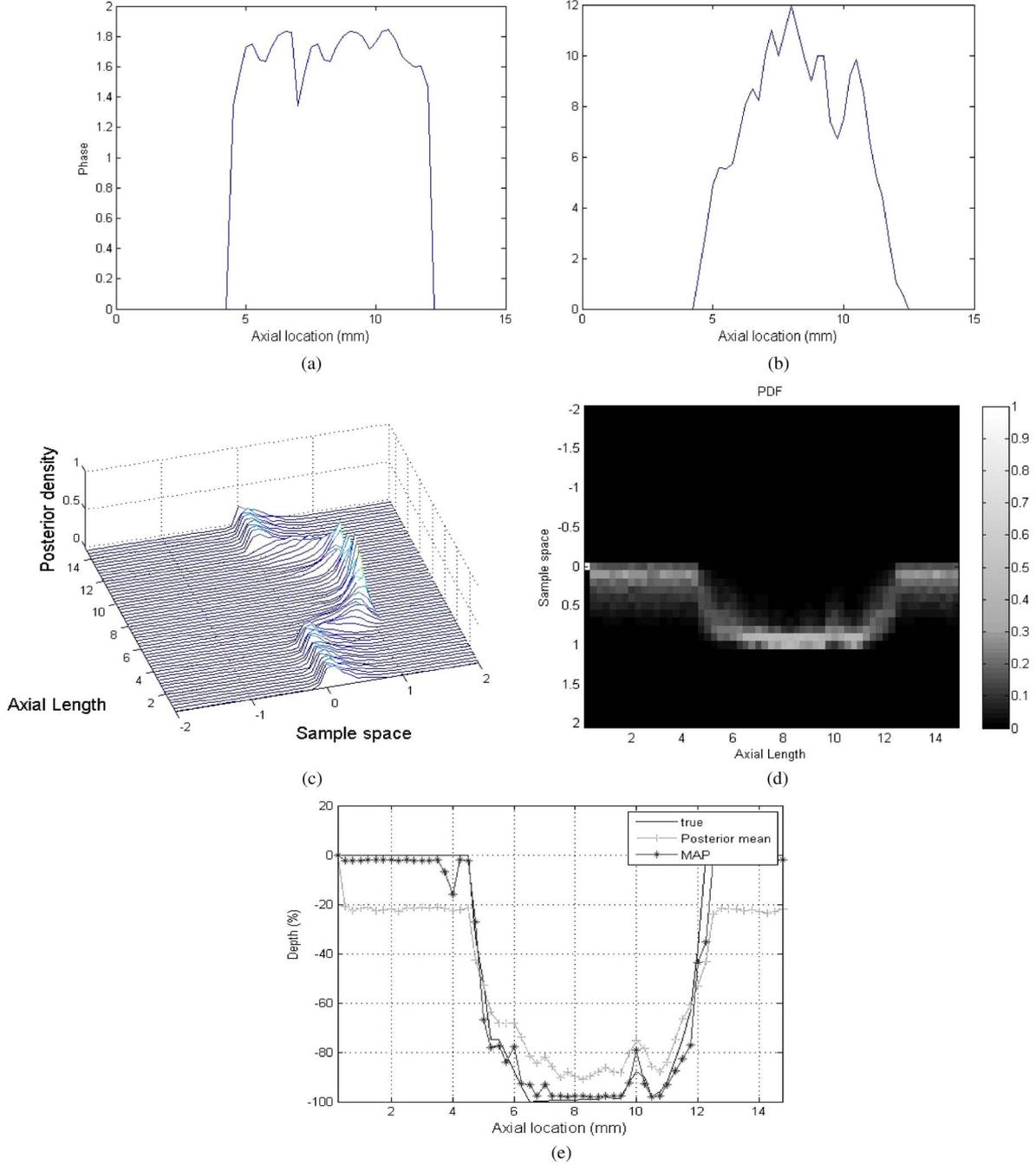
Fig. 5. Proposed inversion technique. (a) Phase measurement. (b) Magnitude measurement. (c) Three-dimensional and (d) top views of the posterior pdf. (e) Computed estimates.
