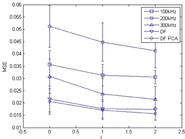
Fig. 7. Mean and standard deviations of the MSE (between the PME and the true profile) versus  $L$  at different measurement modes.
