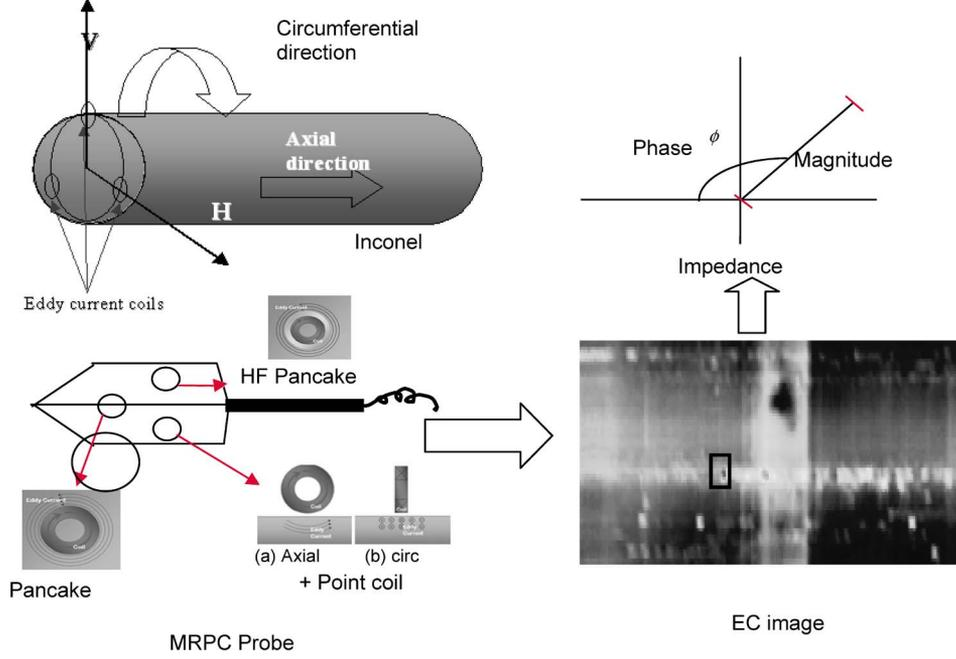
Fig. 4. ECT of steam generator tubing.
