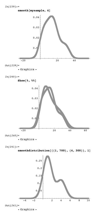
Reproducing the curves of Figure 7.13 produced by smoothing data {84,49,61,40,83,67,45,66,70,69,80,58,68,60,67,72,73,70,57,63,70,78,52,67,53,67,75,61,70,81,76,79,75,76,58,31} according to the method:
